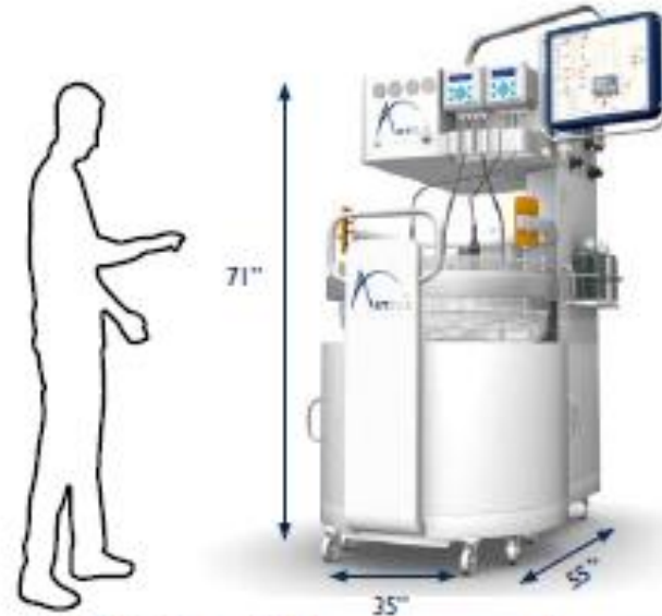
25L iCELLis™ bioreactor mounted on process control skid
